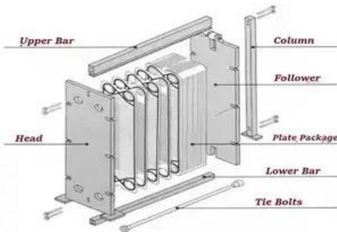
Fig.1 Exploded view of PHE
