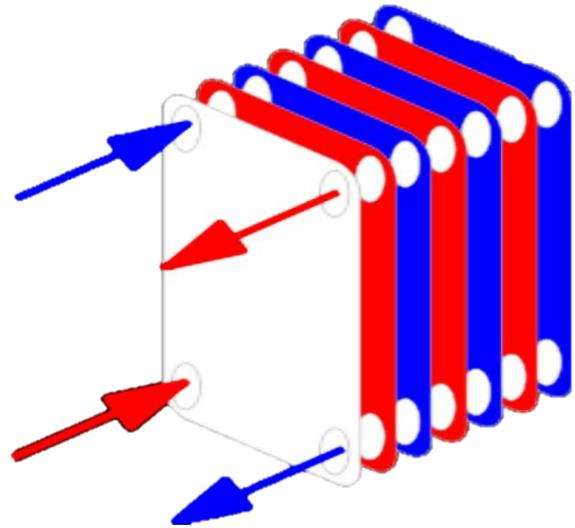
Fig.7 Plate and frame PHE
