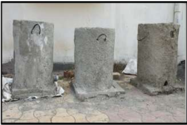
Fig-2 : Constructed Ferrocement Tank
