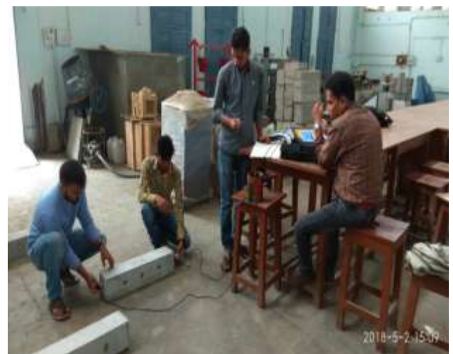
Fig 4: Ultra-sonic Pulse Velocity Test being conducted on GP-PQC specimens
