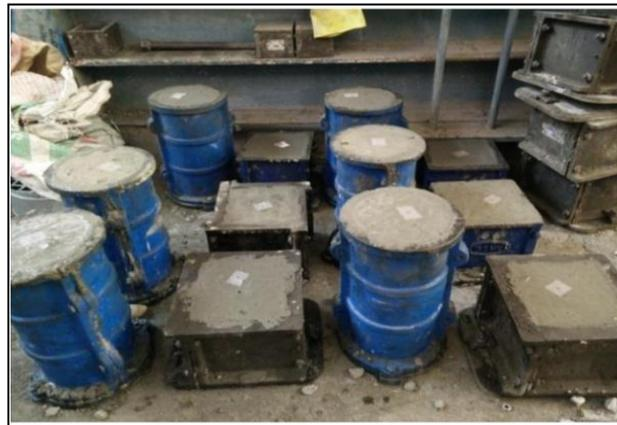
**Fig-4:** Casting of the concrete specimen
