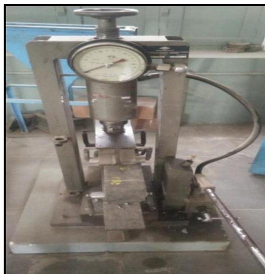
Fig-8: Flexural strength test setup
