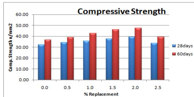
Fig-10: 28 & 60days compressive strength (10M)
