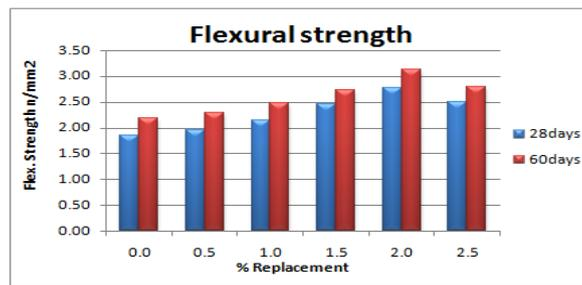
Fig-16: 28 & 60days Flexural strength (12M)
