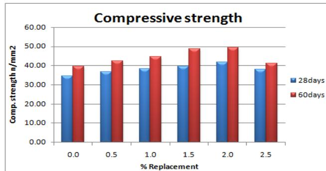
Fig-10: 28 & 60days compressive strength (12M)
