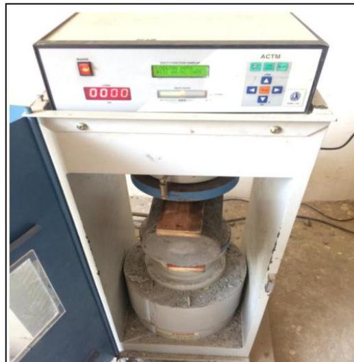
Fig-7: Split tensile strength test setup
