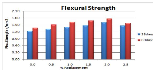
Fig-14: 28 & 60days Flexural strength (8M)
