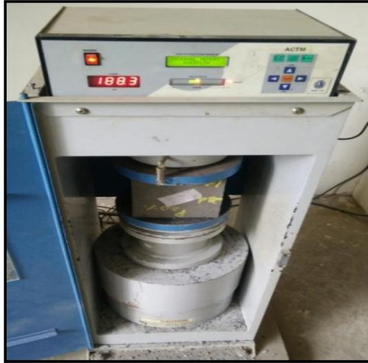
Fig-6: Compressive strength test setup
