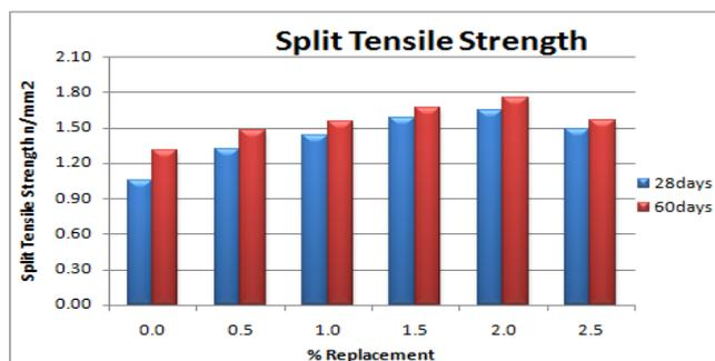
Fig-11: 28 & 60days Split tensile strength (8M)
