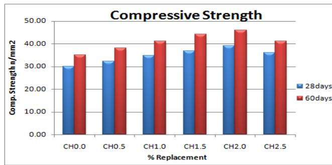
Fig-9: 28 & 60days compressive strength (8M)
