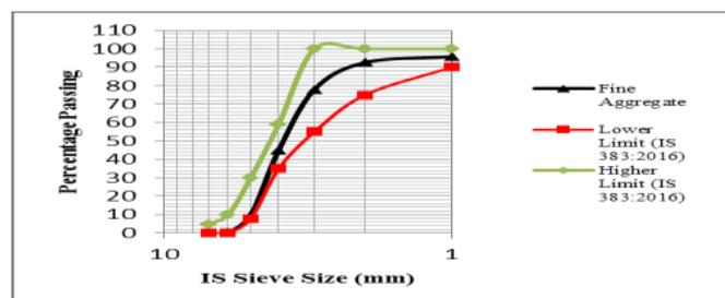
**Fig-1:** Sieve analysis of Fine aggregate
