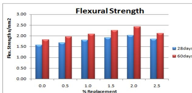
Fig-15: 28 & 60days Flexural strength (10M)
