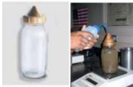
Fig 3.3 . Pycnometer to find out specific gravity
