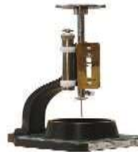
Fig 3 .2 Vicat Apparatus for Consistency, IST, FST.
