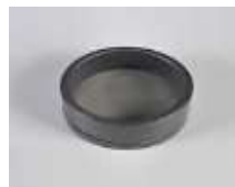
Fig 3. 1. 90 micron sieve for fineness test.
