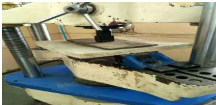
Fig 3.9. Testing of panels for flexure
