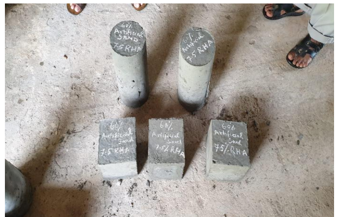
Figure: 2.7 Concrete Cube, Cylinder and Beam Specimens.
