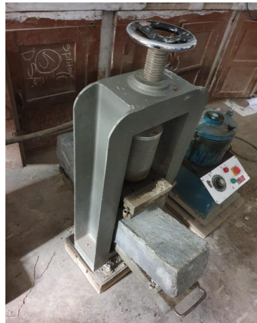
Fig. 2.9 Flexural Strength testing in progress
