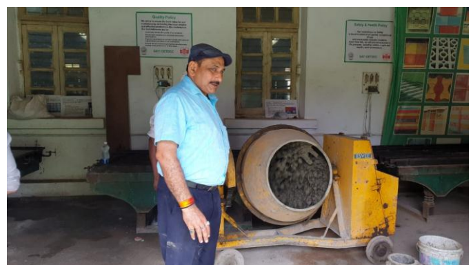
Figure: 2.1 Mixing in concrete mixer
