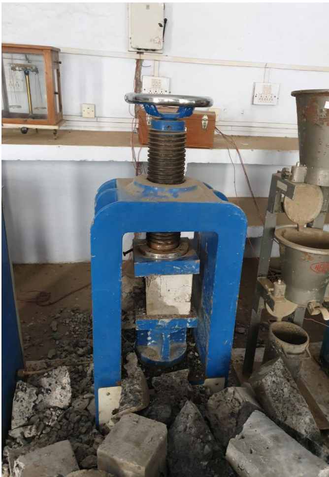
Fig. 2.8 Compressive Strength testing in progress
