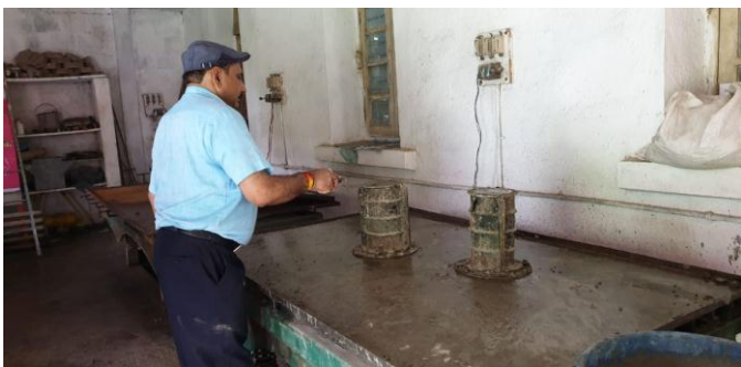
Figure: 2.3 Pouring and Compaction of Fresh Concrete Mix.
