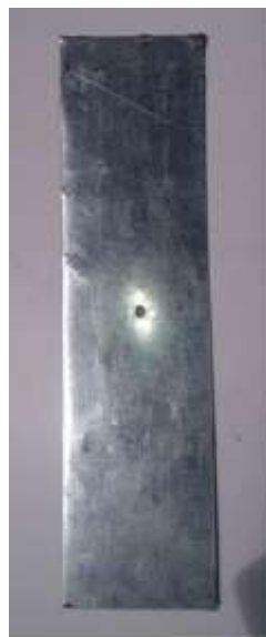
Fig -2.b: Sample specimen work with 50,000 cycle stroke
