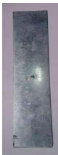
Fig -2.c: Sample specimen work with 75,000 cycle stroke
