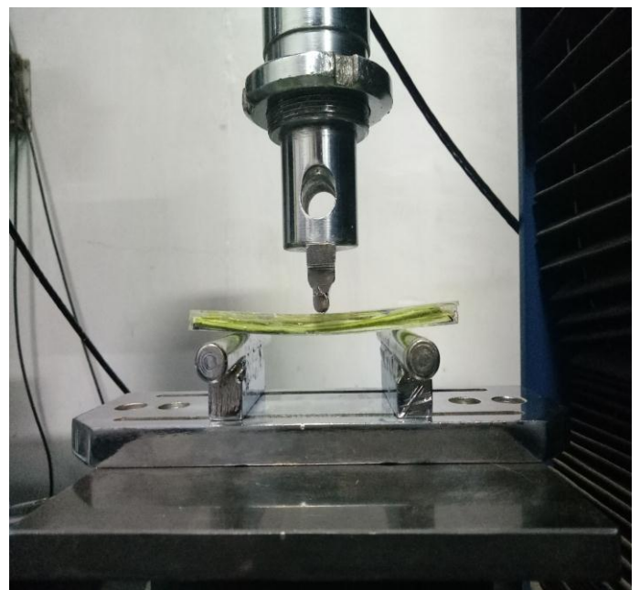
Fig 10: Flexural Testing on UTM machine
