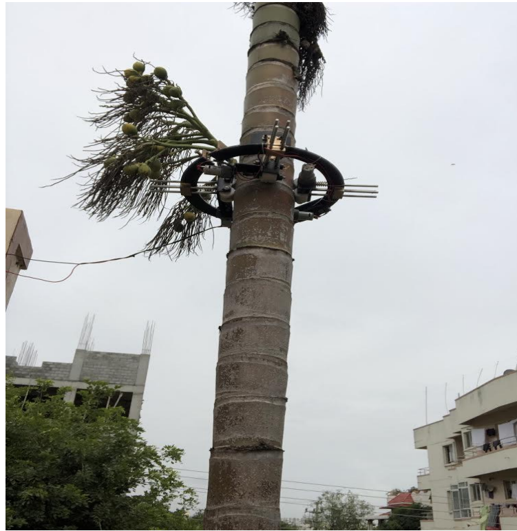
Fig 10 View of Prototype harvesting a areca branch.
