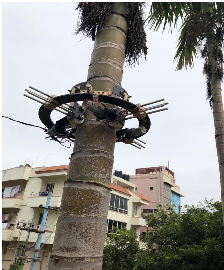
Fig 9 View of prototype climbing a Areca tree
