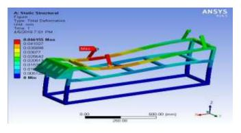
Figure 4: Static structural analysis of frame.
