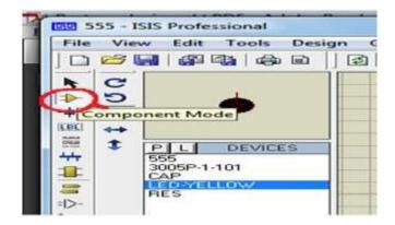
Select the all components from library, that components are added to devices list. Click on the device and change the angle of the device by using rotate buttons. Then click
