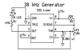
Figure 6.3 Circuit Diagram of 38 KHZ Generator
