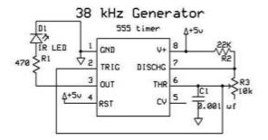
In the above circuit the required components are 555 timers IC, 470? and 22K? Resisters, 10K? Variable resister, 0.001 $\mu$ f capacitor and one IR LED. So select the components from library. In menu bar library > pick device/ symbol. Then one window will open that shown in below.
