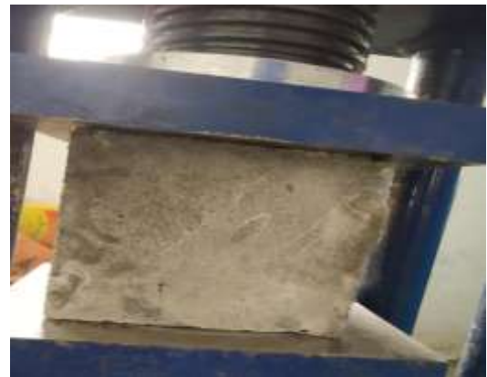
Fig-4: Compressive test
