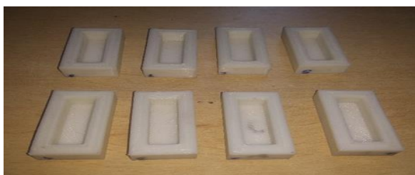
Fig -5: FDM parts for surface roughness and Flatness error measurement
