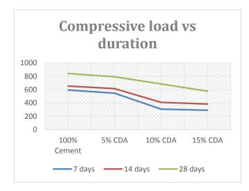
Different cubes of concrete samples were prepared using coarse aggregate and Cement was replaced by cow dung ash (CDA) in different proportions, river sand and potable water was used during preparation of concrete cubes. The cubes were cured for the period of 7 days, 14 days and 28 days. Then the compressive strength of cured samples was determined using Universal Testing Machine.
