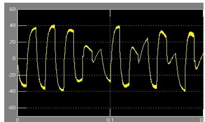
Fig -8: Rotor current characteristics of 1Φ induction motor
