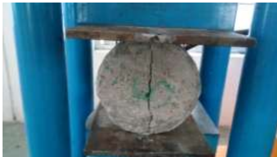
Fig-9: Split Tensile Testing
