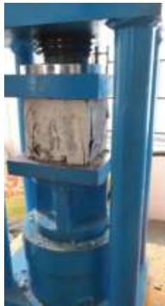
Fig-8: Compression Testing
