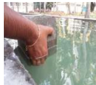
Fig-7: Curing the Specimen
