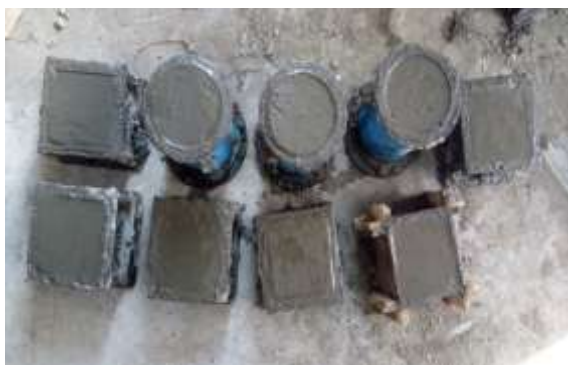
Fig-4: Casting the Mould
