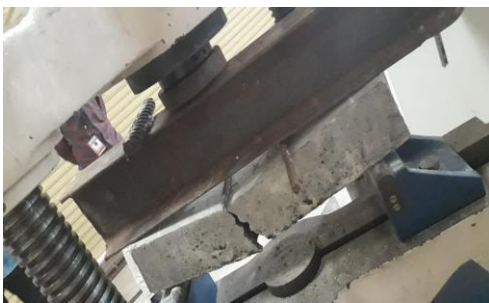
Fig-8 specimen subjected to flexural strength
