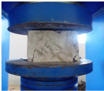
Fig-6 specimen subjected to compressive strength
