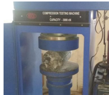
Fig-7 specimen subjected to split tensile strength
