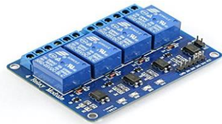
Fig -5: 4-channel relay module
