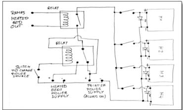
Figure 6: Heat Bed Circuit[11]
