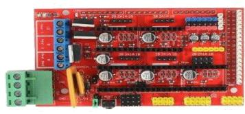
Figure 3: RAMPS 1.4 Control Board
