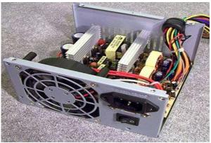
Figure 2: power supply unit
