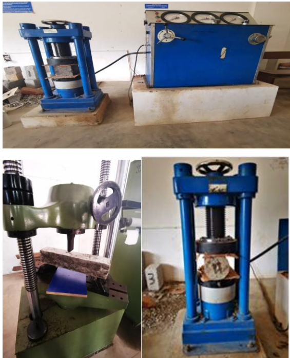
Fig -2: compression testing machine, flexural strength testing machine and split tensile strength testing machine
