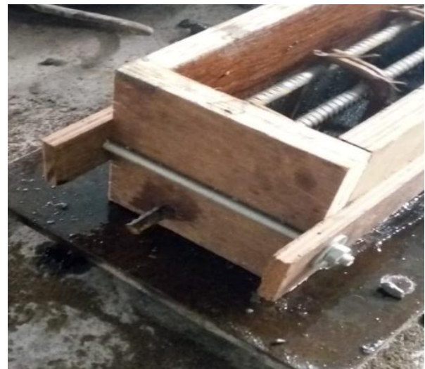
Fig-1: Mould with reinforcement bars
