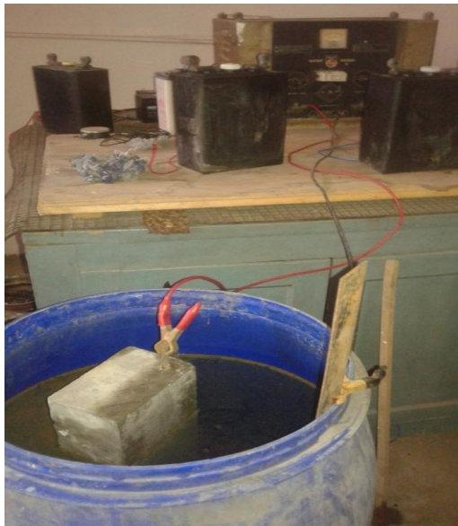
Fig-3: Test setup of accelerated corrosion of beams
