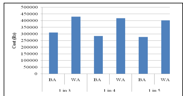
Chart -8: Total cost for varying truss slopes
