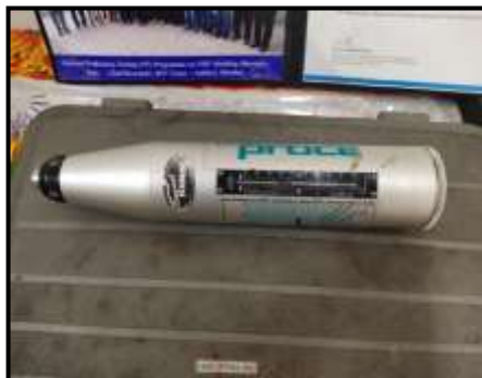
Fig -3: Rebound Hammer Proceq N-34
