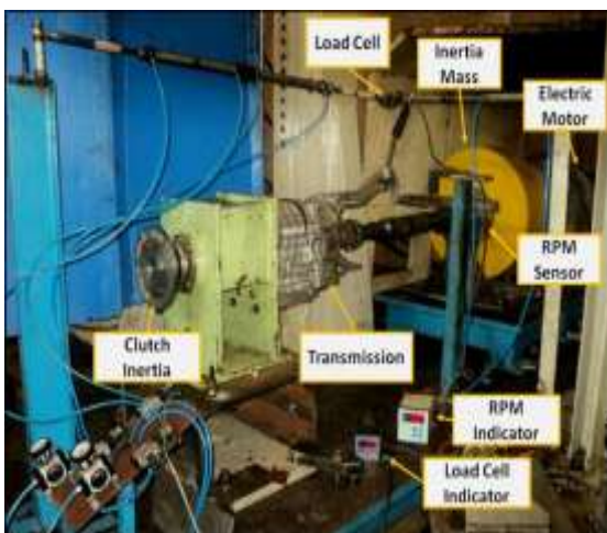
Fig -8: General Setup of Transmission Synchronizer Durability Test
