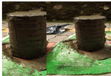
Fig 8: Retrofitting of cylinder
