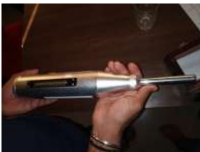
Fig. 3.1 rebound hammer test
