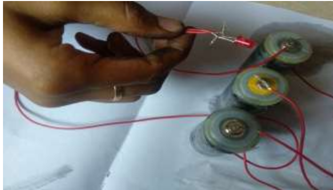
Fig.7.3 led glowing by the voltage produced by series combined dry cells
