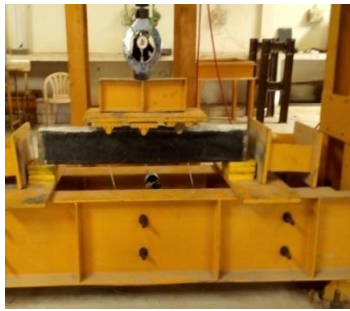
Fig-4: Test Setup for CFRP Beam
