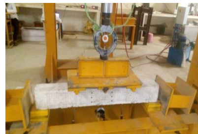
Fig-3: Test Setup for Conventional Beam
