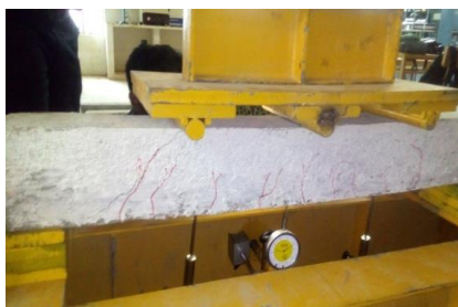
Fig-5: Loading Test on Conventional Beam
