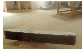
Fig-6 : Three Point Loading Test On CFRP Beam
