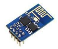
It employs a 32-bit RISC CPU based on the Tensilica Xtensa L106 running at 80 MHz (or over clocked to 160 MHz). It has a 64 KB boot ROM, 64 KB instruction RAM and 96 KB data RAM. External flash memory can be accessed through SPI.
