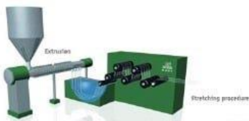
Fig. 6 The stretching of ribs through extrusion process
