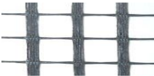
Fig.5 Geogrid sample manufactured by knitting
