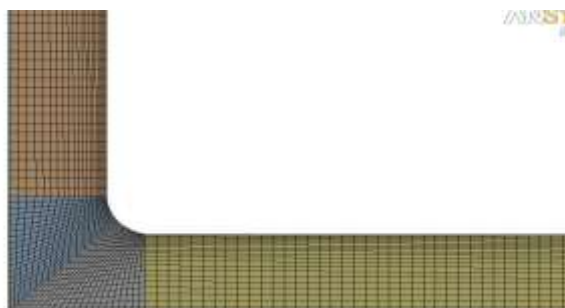
Fig. 4.2 Close View of solar chimney mesh
