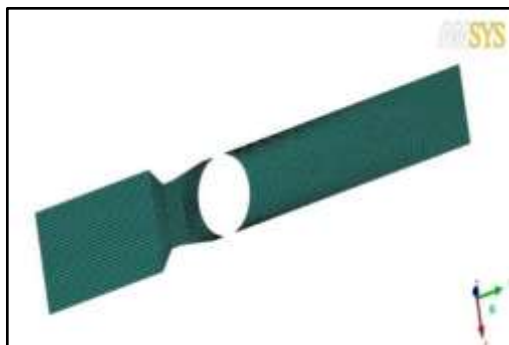
Fig-5: Layer section of structured meshing Venturi with Nozzle and baffle plate.
