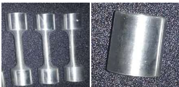
Fig-2: Tensile and Compression Test Specimen
