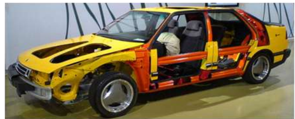
Fig-1: Cross Section of Different Strength of the Metal in a Saab 9000 [4]
