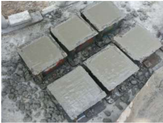
Fig -10: Casting of mortar(1)
