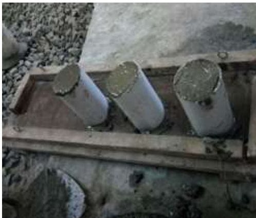
Fig-11: Casting of mortar(2)
