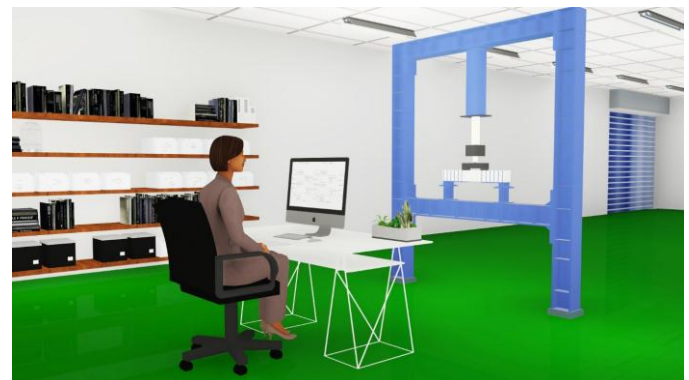
Fig -7: Flexural beam testing scheme on loading frame
