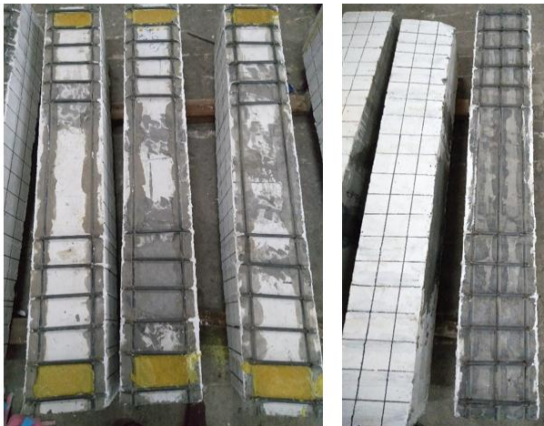
Fig -5: Beams after retrofit with external steel reinforcement method (left 2Ø6, right 3Ø6)
