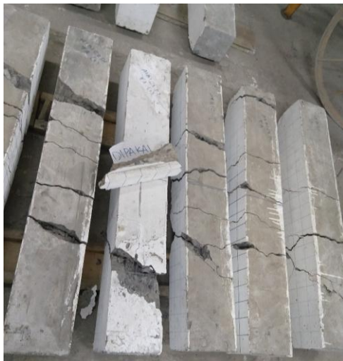
Fig -4: The condition of flexural beam testing after loading up to failure
