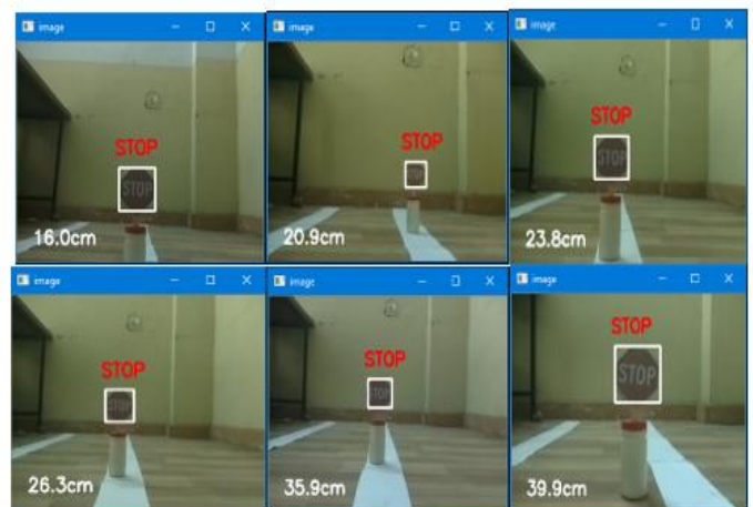
Fig -7: Experimental results of distance measured by Pi camera
