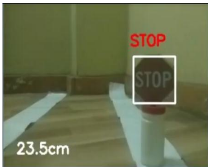
Fig -6: Stop Sign Detection
