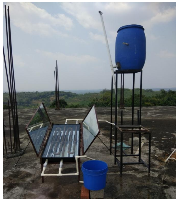
Figure 3.2.1 fabricated solar water heating system
