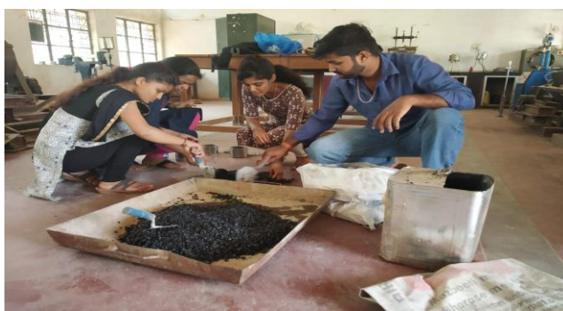
Fig:1 Preparation of Mould for Marshall Tests
