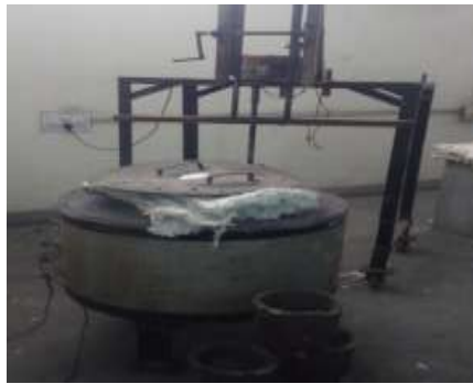
Fig-1: electric arc furnace
