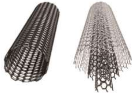
Fig-2. a)Single Walled Carbon Nanotube b)Multiwalled Carbon Nanotube (Source: Toraman et al.,2017)
