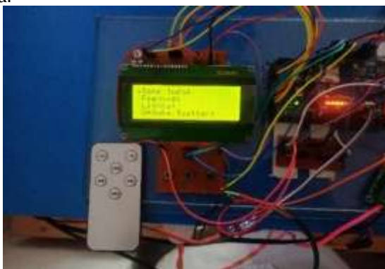
Fig -2: Interfacing Remote to IR sensor
