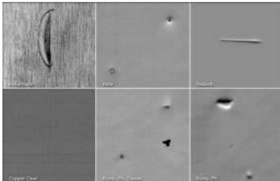
Fig 4.1: Different types of cracks
