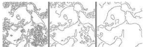
Fig 8.3: Edge detection by Canny method (sigma=1,2,3, T1=0.3, T2=0.7)
