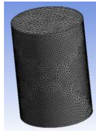
Fig. 5.2 - Meshing of optimized piston
