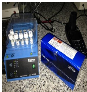
Figure 10 COD Thermo -Reactor & COD meter
