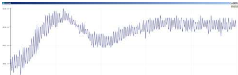
Fig- 4: Flex sensor 2 bent at 90 angle
