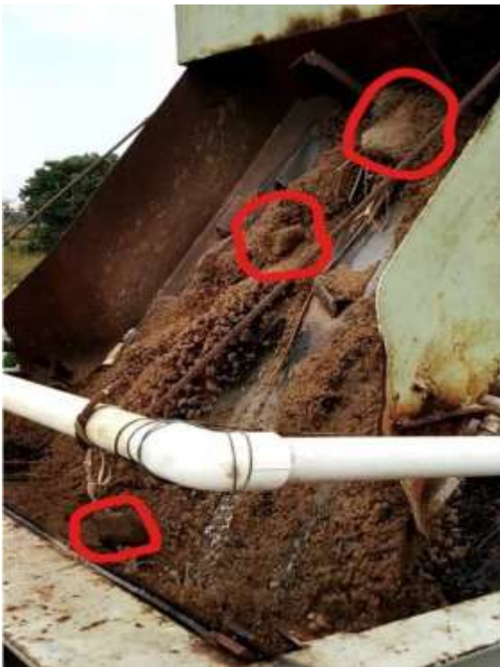
Fig 2. Heavy stones in primary screener
