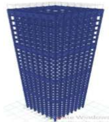
Fig- 5: 30 Storey building with outrigger system
