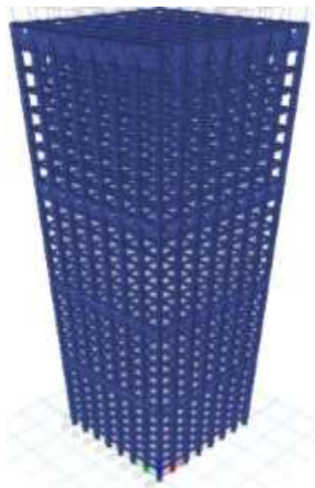
Fig- 8: 30 Storey building with outrigger system
