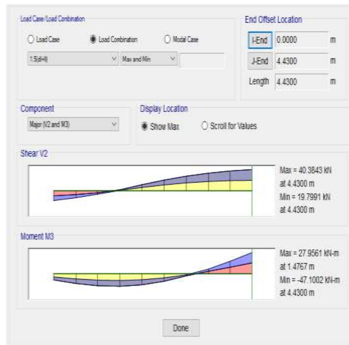
Fig-4 : Maximum and Minimum Bending Moment And Shear By E-TABS
