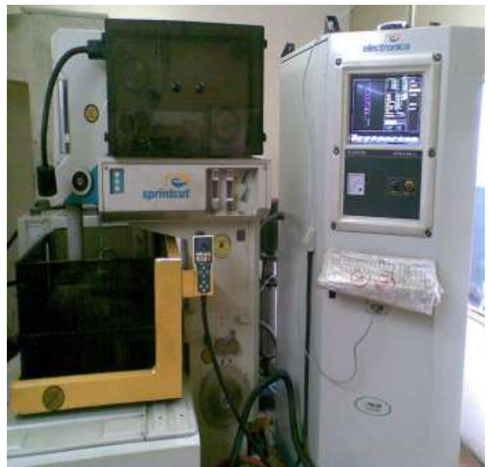
Figure 2.3: Experimental set-up of wire cut EDM [Courtesy NSIC, Aligarh (India)]
